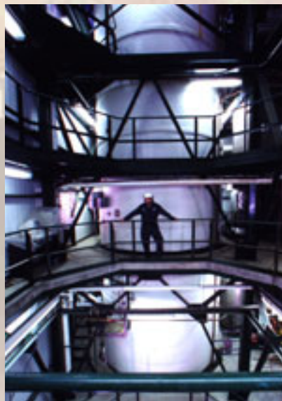
The fermentor: Tank used to process the sugars into what the industry calls "beer." This is then distilled into alcohol (ethanol).
