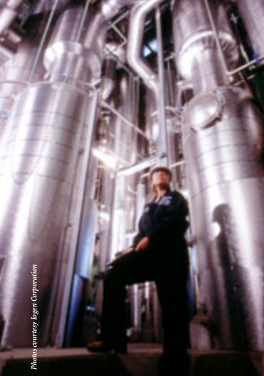
The evaporator: Concentrates the fermentable sugars and the "still bottom" (residue) from the fermentor after the sugars are fermented into "beer."
